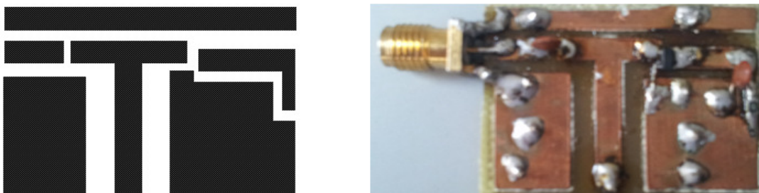
Fig 5. Layout and fabrication of rectifier.
