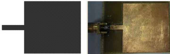
Fig 8. Layout and fabrication of the antenna.
